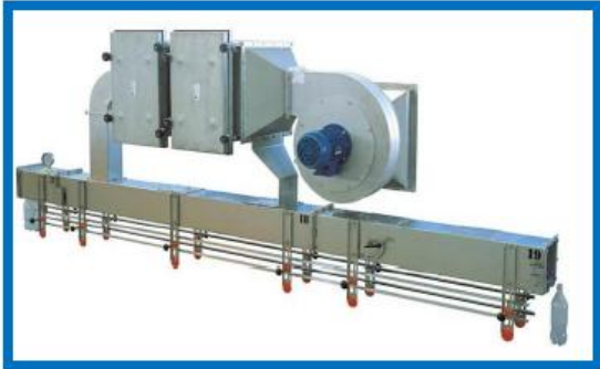
Air conveyor for PET bottles
